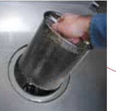
Pre-Wash table Easy removable filter system
